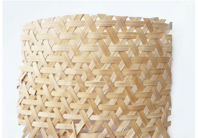
竹编三叉 Bamboo woven three forks 网孔直径Diameter of mesh10mm
